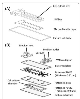
**Fig. 1** Design of the custom-fabricated microfluidic device. **a** Schematic representation of the "pre-culture well". **b** The assembly of the microfluidic device with a cross-sectional view of the structure. *PDMS* Polydimethylsiloxane, *PMMA* Polymethyl methacrylate
