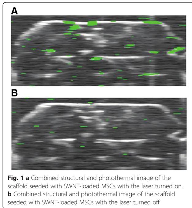
**Fig. 1** **a** Combined structural and photothermal image of the scaffold seeded with SWNT-loaded MSCs with the laser turned on. **b** Combined structural and photothermal image of the scaffold seeded with SWNT-loaded MSCs with the laser turned off
