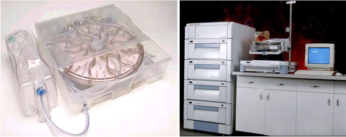
Figure 1. Astrom manufacturing platform. Left: single-use cell cassette. Right: highly automated instrument platform.
